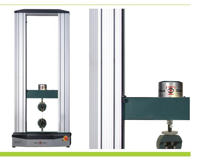
The 50ST Loadcell above crosshead model is a variation of the Tinius Olsen 50ST Electromechanical Materials Testing Machine. It is a robust design for use in a range of materials testing.
