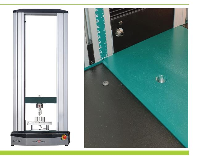
The 50ST dust & particle ingression resistance model is a variation of the Tinius Olsen 50ST Electromechanical Materials Testing Machine. It is a robust design for use in a range of materials testing.
