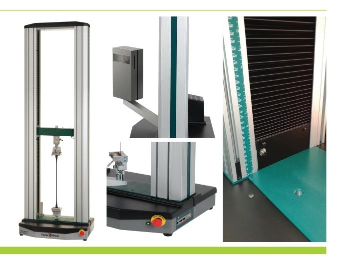
The 25ST Extended height model is a variation of the Tinius Olsen 25ST Electromechanical Materials Testing Machine. It is a robust design for use in a range of materials testing.
