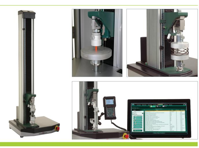
The 1ST extended model is an Electromechanical Materials Testing Machine. It is a robust design for use in a range of materials testing.
