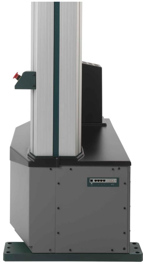
The 150ST Extended height model is an Electromechanical Materials Testing Machine. It is a robust design for use in a range of materials testing.
