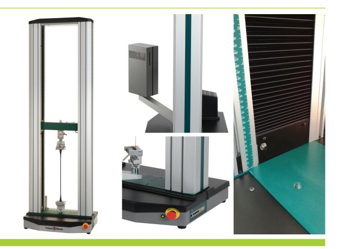
The 10ST extended height model is an Electromechanical Materials Testing Machine. It is a robust design for use in a range of materials testing.
