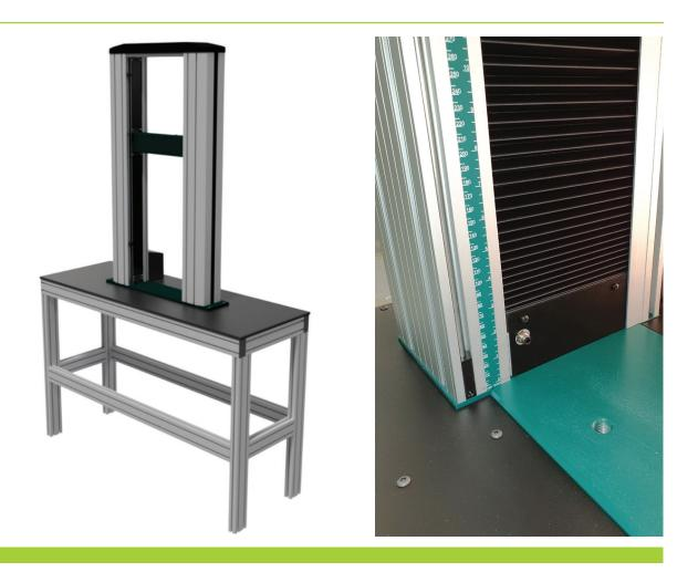
The 10ST base enclosure mounting model is an Electromechanical Materials Testing Machine. It is a robust design for use in a range of materials testing.
