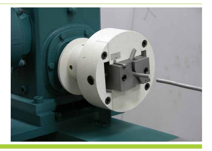
The Tinius Olsen wire twisting machine is a benchtop system that provide the simplicity, performance and affordability needed for quality control and product testing.
