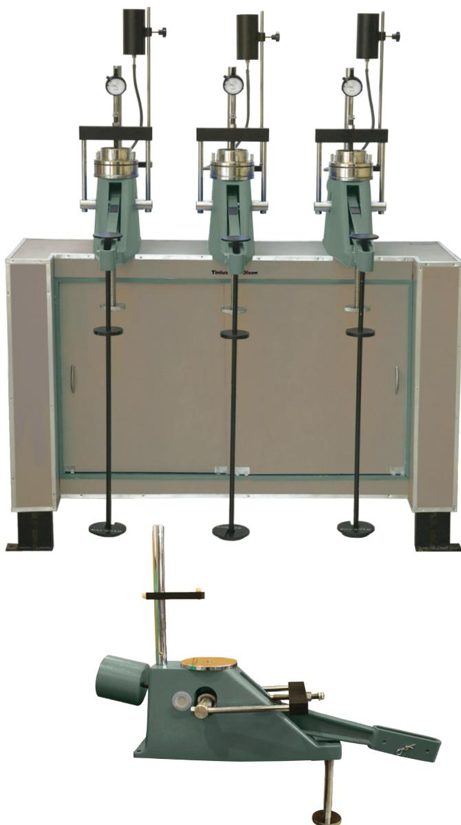
The Consolidation Apparatus consists of a fixed ring type of consolidometer cell for testing specimens of 60mm dia x 20mm thick, but a variety of specimen sizes from 50 to 100mm dia can also be tested. Additionally, the same loading unit can be used with optional floating ring consolidometer cells.
