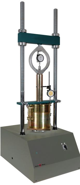
The California Bearing Ratio test (usually called CBR test) is an empirical test developed in California, USA. It determines the relative bearing ratio and expansion characteristics under known surcharge weight of base, subbase and sub grade soils for the design of roads, pavements and runways. The CBR test is used extensively in selection of materials and control of sub grades.
