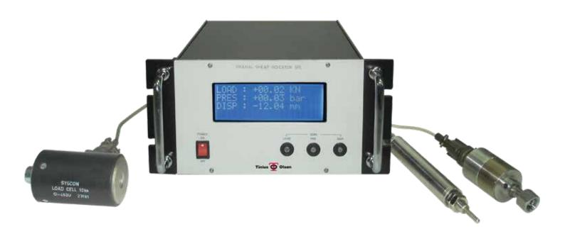
he Triaxial Data Acquisition System comprises a 10kN (1000kgf) capacity external load cell, a 20 bar (20kg/cm) capacity pore pressure transducer, an LVDT displacement sensor with a range of ±10mm, and a 3-channel digital indicator that has been specially designed to meet the requirements of triaxial testing.
