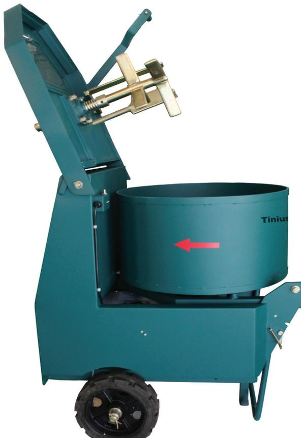
For quality specimens to be manufactured, efficient mixing of concrete prior to molding is essential. Efficient mixing helps by coating the surface of all aggregate particles with cement paste and also creates uniformity in the mixture. The pan model is suitable for mixing small quantities of concrete, typically used in laboratories.
