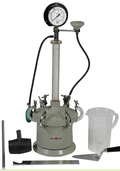
ntrainment of a small amount of air in cement concrete has been found to considerably improve the durability of concrete. The recommended limits specified for the air content are between 3% and 6.5%. Smaller percentages may result in deterioration taking place more quickly and larger percentages may reduce the strength without any improvement in the durability of concrete.
