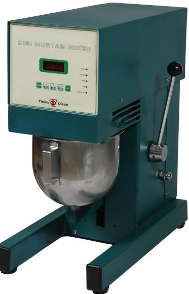
his mixer is designed to mix mortars and cement paste to standard requirements and can be operated in either manual or automatic mode.
