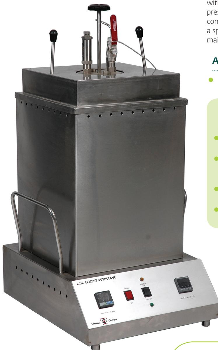
The Cement Autoclave is ideal for conducting accelerated soundness tests on cement and consists of a stainless steel pressure vessel with insulated outer shell. The temperature and pressure are measured by RTD probes and the system controlled by a PID controller, but the system has a spring-loaded pressure release safety valve to maintain safe operation.
