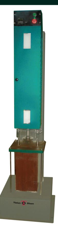
he Automatic Compactor eliminates the laborious process of manual compaction and results in consistent laboratory specimens.
