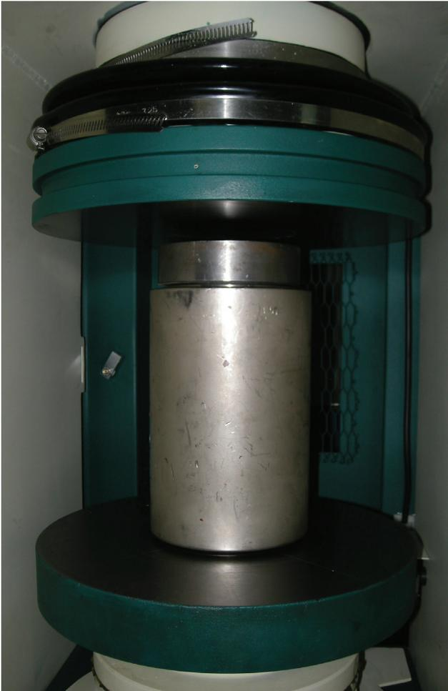
BS EN 12390 requires certified stability and alignment, which is achieved using an oil-filled ball seating and upper platen.
