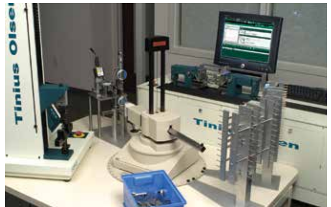
Detail showing the pick-and-place robot, sample racks, laser barcode reader, sample dimension measuring station, broken sample bin and another test station. This second test station could be flexure, hardness or another kind of physical test
