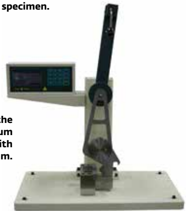
Model IT504 – In this configuration, the machine has been equipped with cold box (top cover removed). Liquid nitrogen is the typical medium used to cool the specimen.
