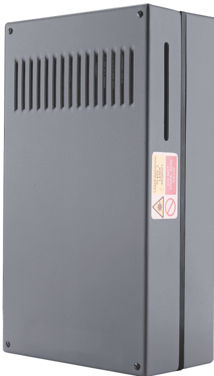
Model 500LC scanning laser extensometer.
