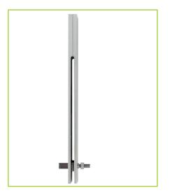
Double shear bearing strength test comprises two loading plates which are secured to the test specimen using a high tolerance, lightly torqued fastener. The fixture is used with upper and lower tensile wedge grips.
