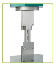
Single shear bearing strength test for use in compression or tension as required.
