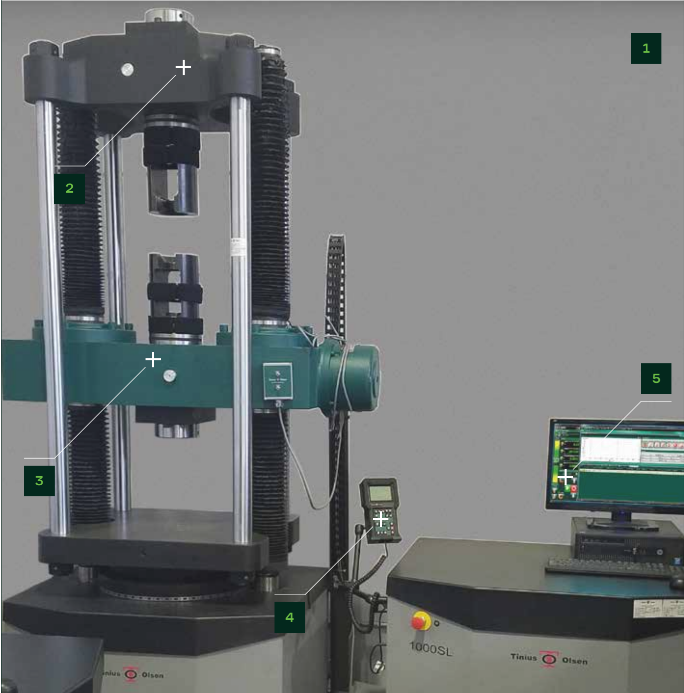
1,000SL rack & pinion crosshead[09009400] with Slotted bolt holder [01031003] and Horizon software [21001197]
