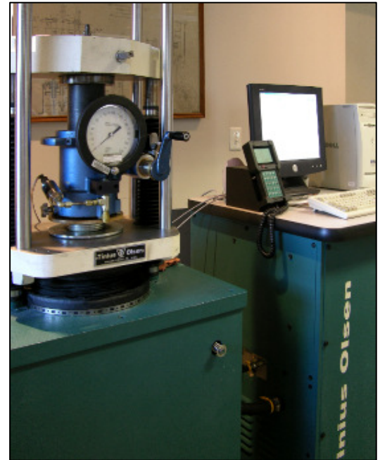
Fig 1. Typical system configuration using a modified stabilometer and Test Navigator software
