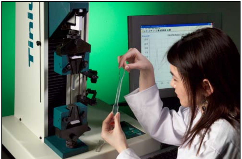
Fig 1. Plastic tensile specimen about to be tested in single column tensile tester, shown with long travel extensometer
