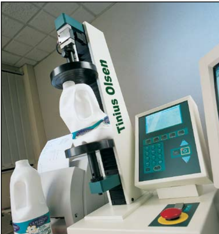
Fig 4. Single column low force tester testing the compressive strength of plastic milk containers.
