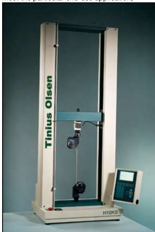
Fig 2. Twin column tensile tester, with a maximum load capacity of 2,200 lbf (10kN), shown testing some plastics strapping material.
