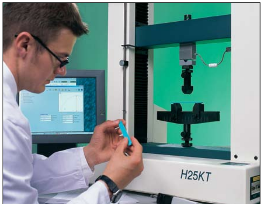
Fig 6. Flexural test on a reinforced plastic specimen.
