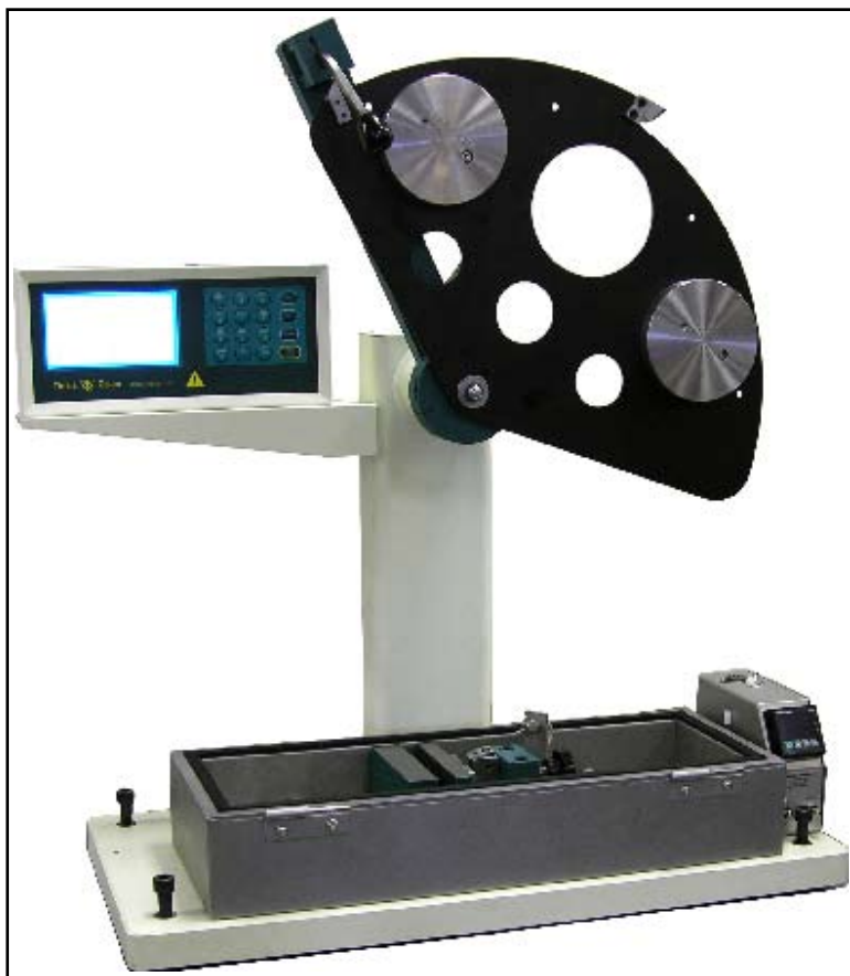
Fig 3. Tinius Olsen's model IT504 impact tester, configured for Izod testing, shown with a cold box to reduce the test temperature (the lid is removed for this picture).
