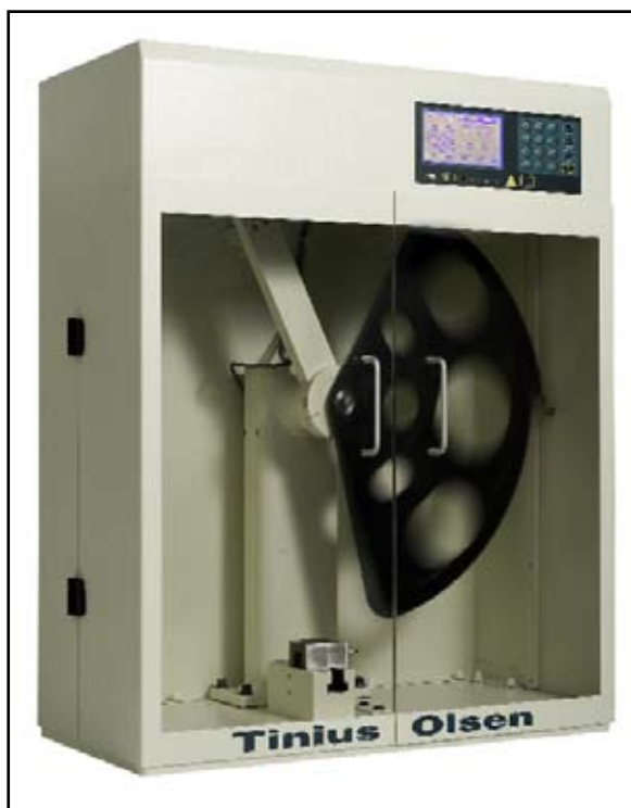
Fig 2. Tinius Olsen's model IT503 enclosed impact tester, capable of performing both Izod and Charpy impact tests on plastic specimens, with up to 25J of available energy with add-on weight sets.
