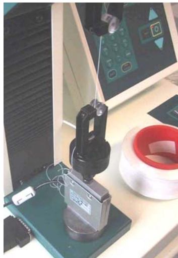
HT58 Bottom Grip with 5N Loadcell and Damper Attachment
