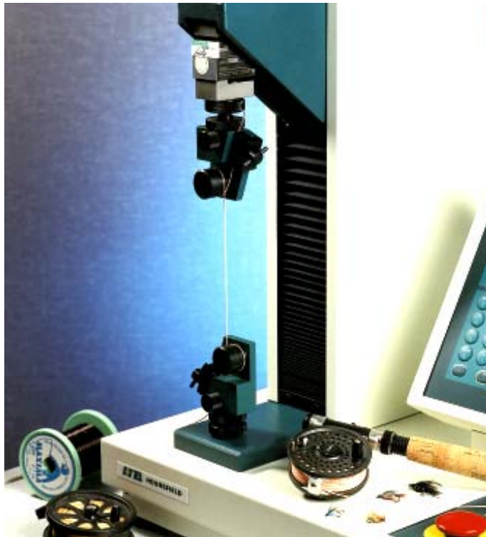
Fishing line assembled in HT33 attachments, ready for tensile test
