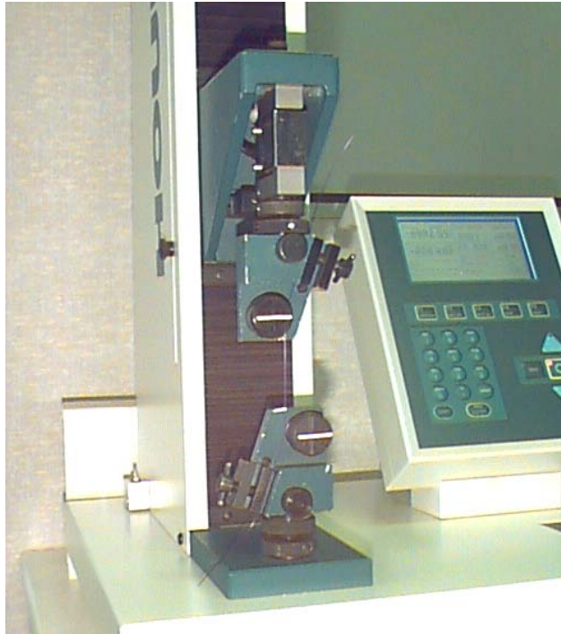
Suture Medical thread assembled and ready for test
