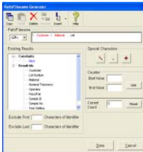
Screen 10. This screen shows the flexibility of the import capabilities of Test Navigator Plus. Here is where the import data is obtained, based on user-defined criteria.
