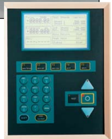
Fig 3. Console of H75kS machine in numerical display mode. Connection to a pc and / or printer is made through the console.
