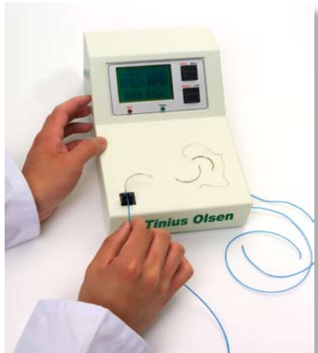
Fig 1. Testing sutures is just one of the many applications of the LF100.
