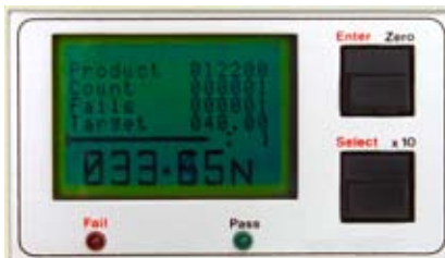
Fig 3. Display indicating one test at a target value of 40N with one failure – main display shows this failure at 33.65 N
