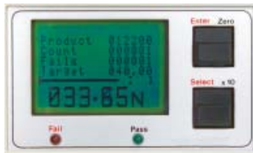
Fig 3. Display indicating one test at a target value of 40N with one failure – main display shows this failure at 33.65 N
