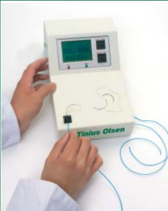
Fig 1. Testing sutures is just one of the many applications of the LF100.
