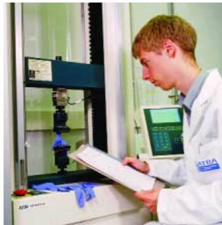
SATRA's H100KS is in regular use for testing PPE
