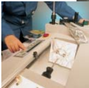
Fig 6. Model H5kW being used to test crimp connectors
