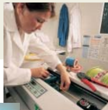
Fig 6. Model H5kW being used to test crimp connectors
