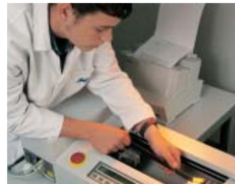
Fig 8. Model H20kW being used to find the tensile strength of steel strips
