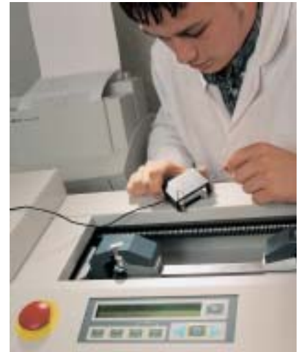
Fig 1: Model H5kW shown with low cost wedge grips
