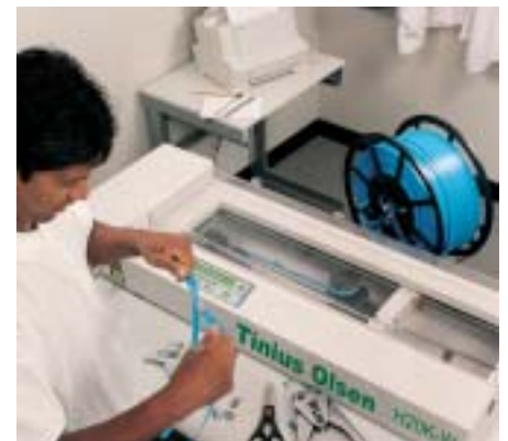
Fig 5: Model H20kW being used to determine the strength of plastic strapping
