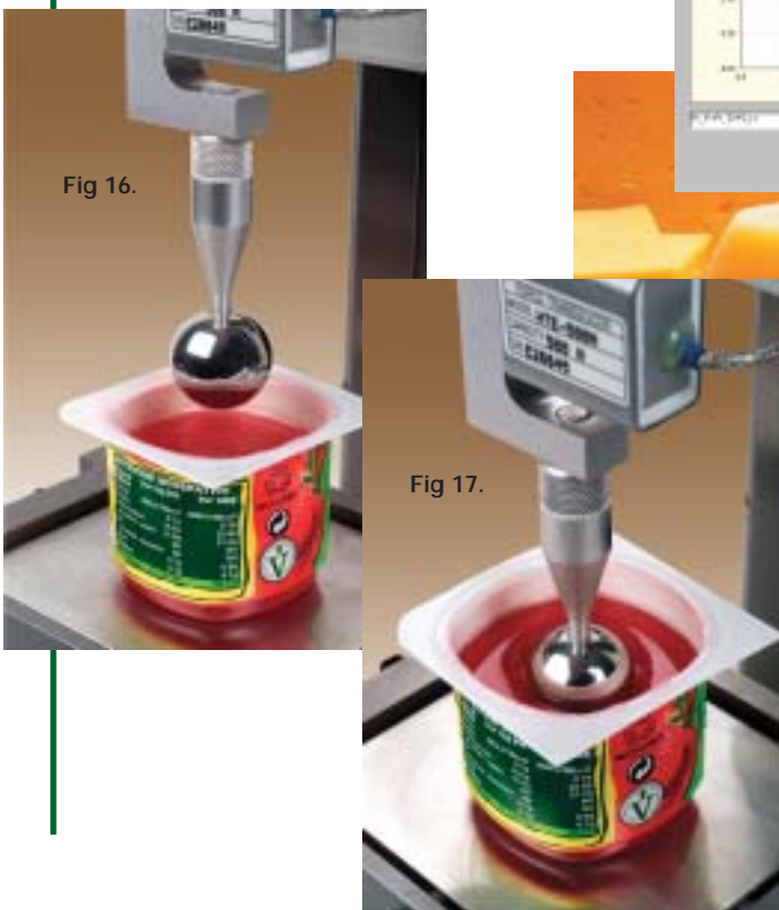
Fig 16 and 17. Before and after photos of a ball probe being used to determine the softness of a gelatin based pudding.
