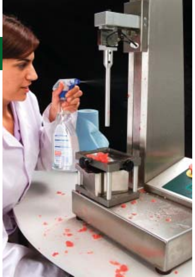
Fig 1. Food tester being cleaned with water after testing. The surgical grade stainless steel construction of the food tester makes this possible without damaging the machine.
