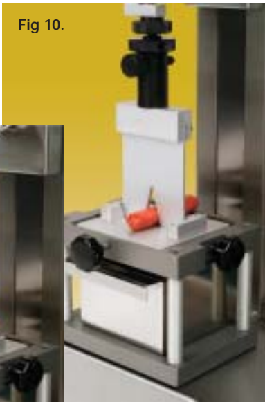
Fig 10 and 11. Before and after shots of a frankfurter being sliced in a Warner Bratzler shear cell.
