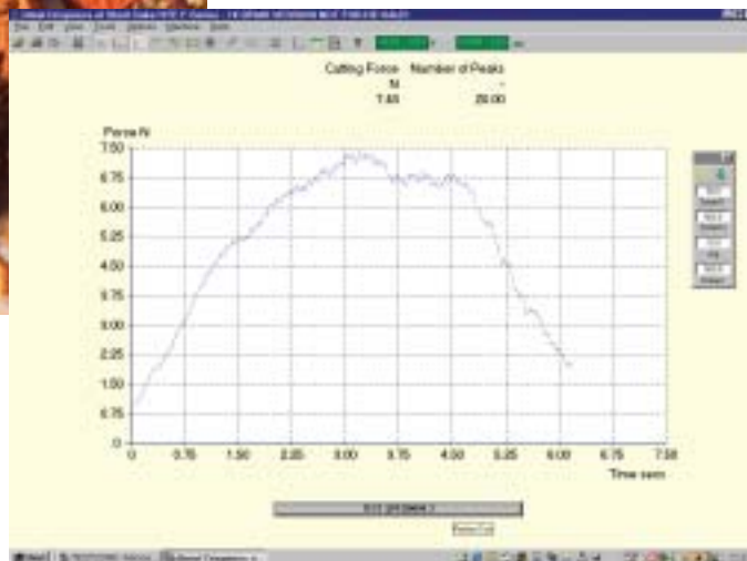
Screen 4. Test profile of a crisp, or potato chip, being crushed with a ball probe.
