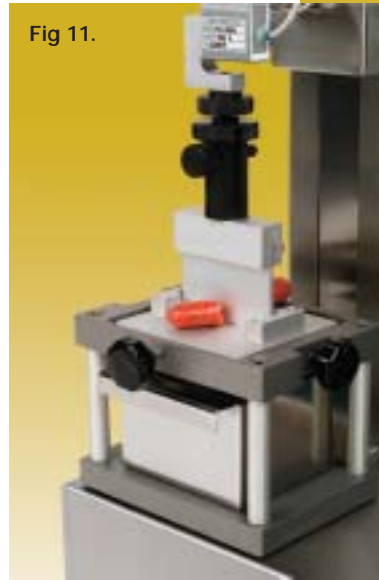
Fig 10 and 11. Before and after shots of a frankfurter being sliced in a Warner Bratzler shear cell.
