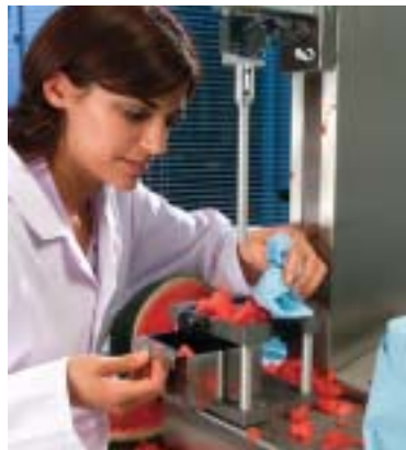
Fig 3. Puncture probes are used to determine the ripeness of various fruits. Here you can see the simple collection tray after testing some ripe watermelon.
