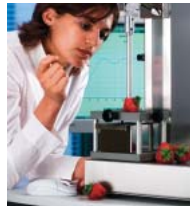
Fig 5. Large and small fruits and vegetables can be tested on the sample test platform. This platform has a holed insert table with a product collection tray located underneath.
