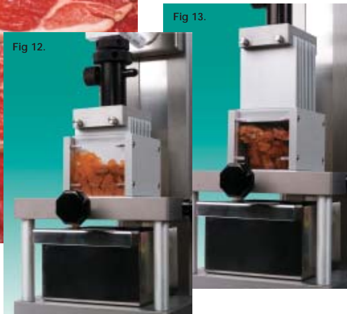
Fig 12 and 13. Before and after shots of cat food being checked with a Kramer Shear Cell.
