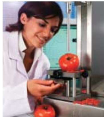
Fig 4. Both fruits and vegetables can be tested, such as the tomatoes shown here, and any spray from the samples can be simply washed off.
