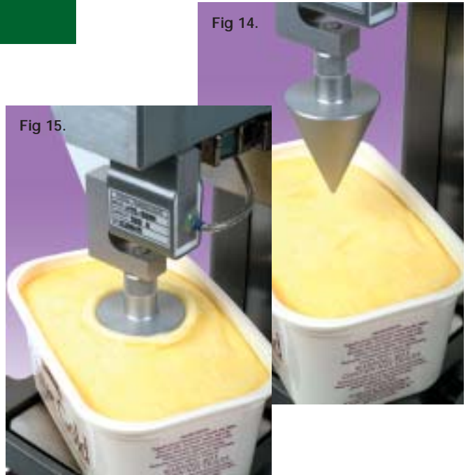
Fig 14 and 15. Before and after shots of a conical probe being used to determine the spreadability of margarine.
