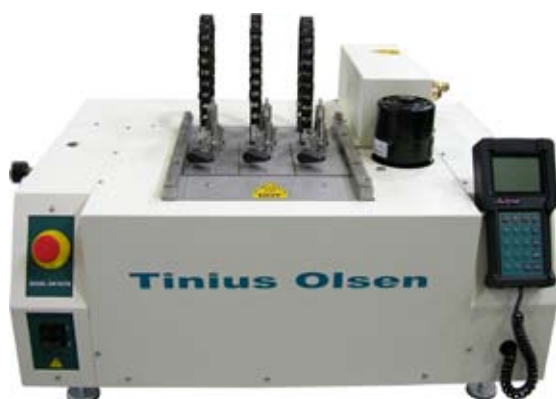
Fig 2. Model 303 HDTM shown with optional third test station, for deflection temperature and / or Vicat testing. Model here shown with three stations, gantry lowered, and optional cooling connections.
